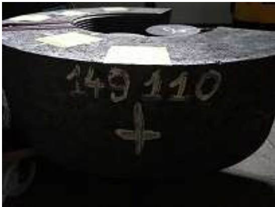
Figure 46 – Measurement of electrical conductivity on different areas on the "270 °" reference block by ConducSens (tm)
